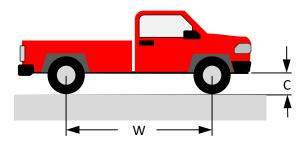
To avoid hangups, measure wheelbase and underclearance of vehicle and check with us.
